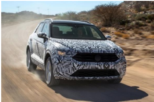
Figure 3.8 - T-Roc on road test with a specific paint to hide the design
