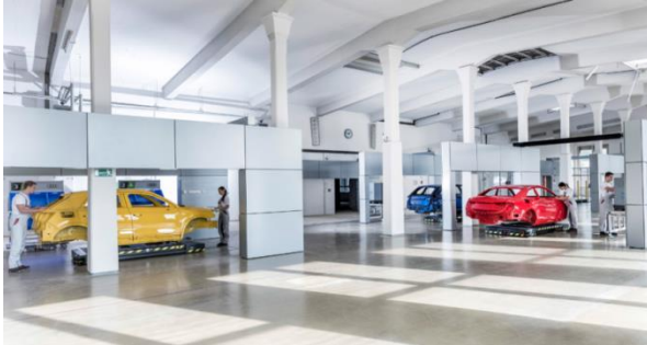
Figure 2.12 - Audi's Modular Assembly Line
